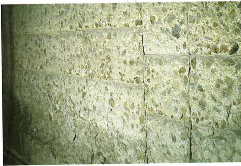
Fig. 5 Precast cooler wall blocks after two years in service (Courtesy of Wahl Refractories)
