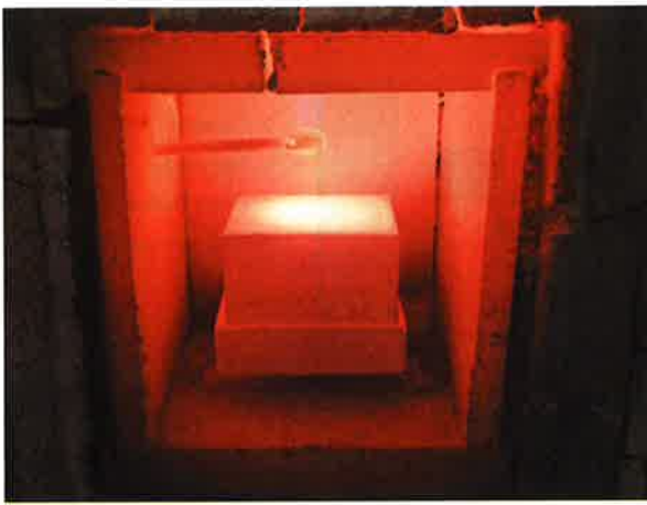
Fig. 5 Thermal shock testing method using open-flame burners.
