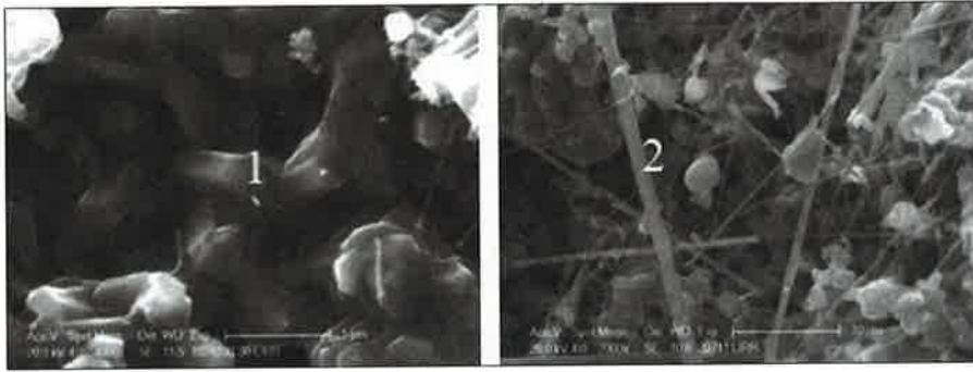
Fig. 1 In-situ generated hexagonal and fibrous SiAlON crystals in SiC-based castable nitrified at 1420 °C (Si powder addition: 7 %)
